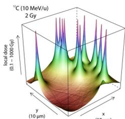
Figure 2: Local dose deposition pattern for Carbon ions at a typical clinical dose.
