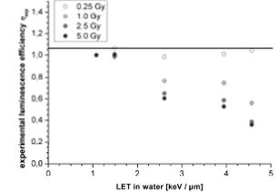
Figure 2: Example of relative RL efficiency dependent on LET and dose (measured at PSI proton beam-line).
