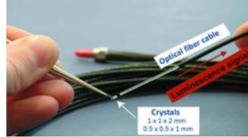
Figure 1: Fiber dosimeters with Al<sub>2</sub>O<sub>3</sub>:C single crystals.
